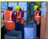
Screening process where the glass bulb is separated from the glass mount/support.
